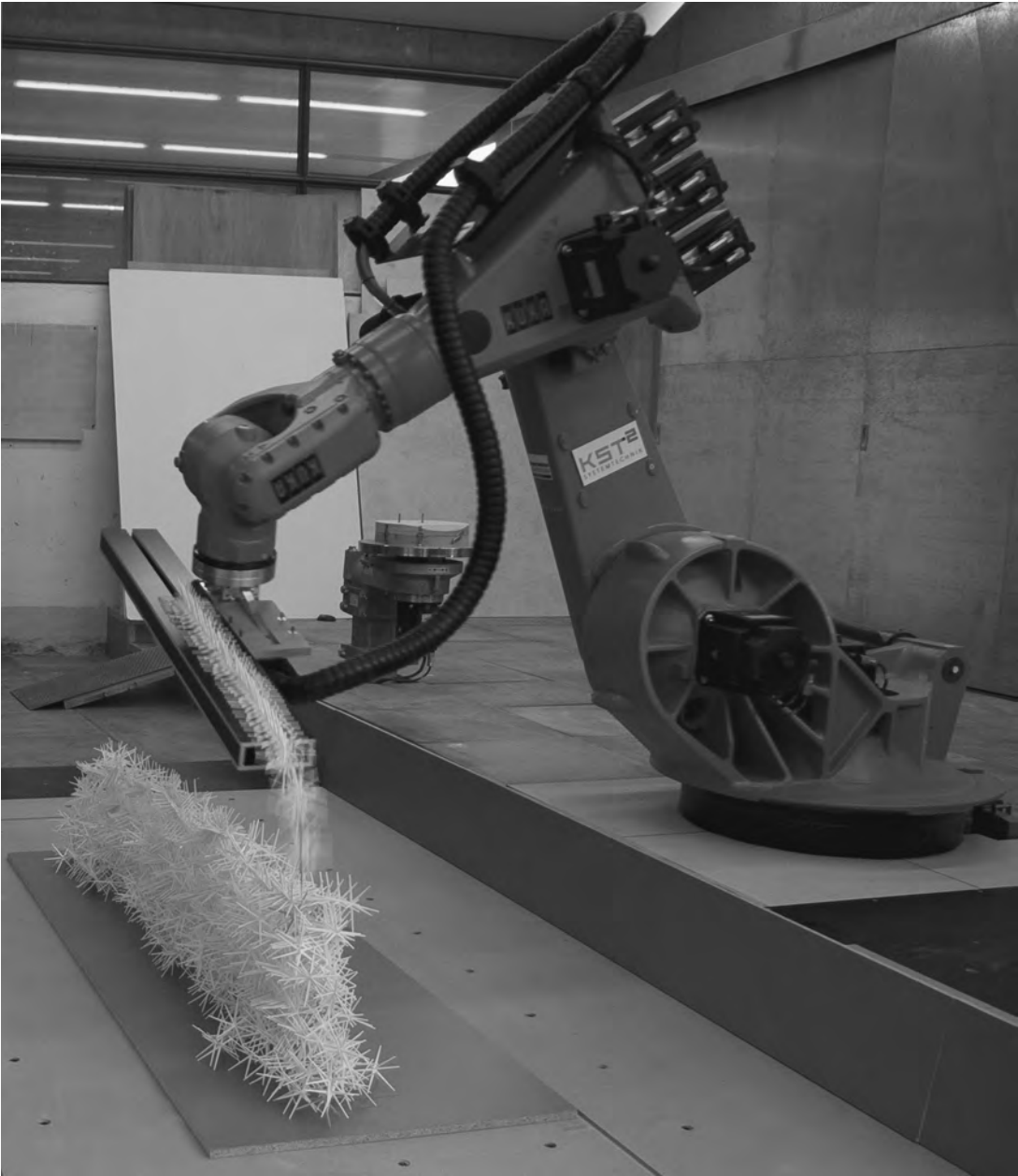
FIGURE 1.11. Aggregate Architectures , by Karola Dierichs, Institute for Computational Design, University of Stuttgart, 2011. A six-axis industrial robot pours out loose components into prespecified shapes. Owing to the components' morphological design, gravity and surface tension hold them together to create the architectural form.
