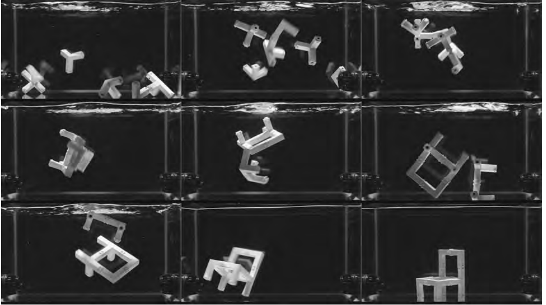
FIGURE 2.1. Fluid Assembly: Chair , by MIT's Self-Assembly Lab with Baily Zuniga, Carrie McKnelly, Athina Papadopolou, and Skylar Tibbits in collaboration with Arthur Olson and Autodesk Inc., funded in part by MIT's International Design Center, 2014. This project entailed the design of uniquely differentiated parts that fit only one place in the final chair. Over seven hours, turbulent water in an aquarium jostled the parts until they joined together into the structure. Tibbits refers to this as "autonomous assembly" and states that it "points towards an opportunity to self-assemble arbitrarily complex differentiated structures from furniture to components, electronics/devices, or other unique structures."
